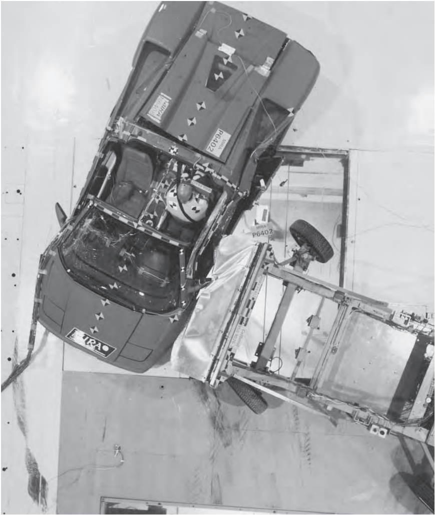
Fig. 36.5 View from above of an impact test in which a sled, on which is mounted a dummy front end, is propelled towards the side of the target vehicle
