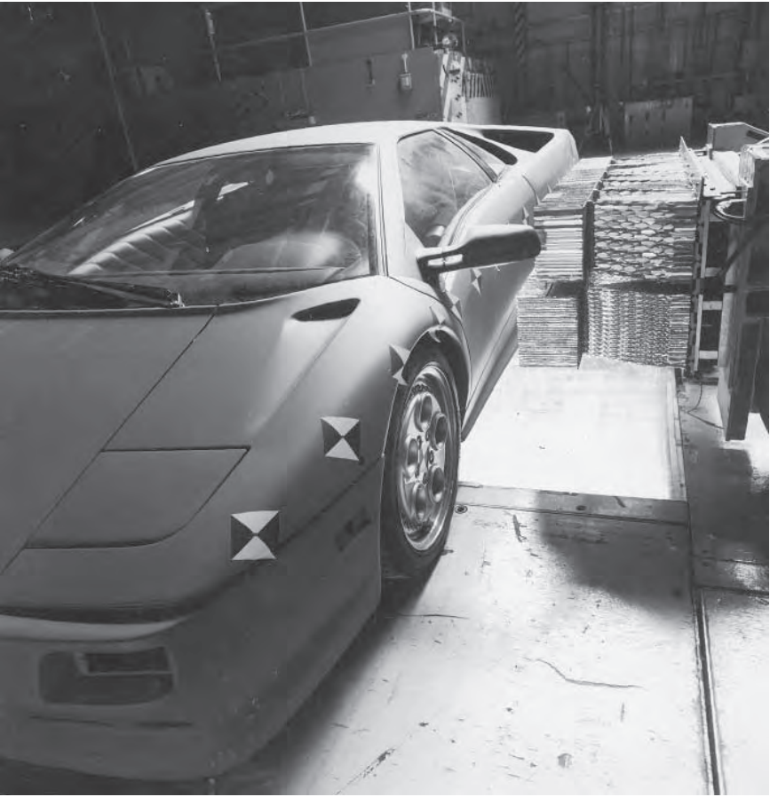
Fig. 36.4 This aluminium honeycomb used in a side impact test is profiled to represent the vertically varying stiffnesses of the other car
