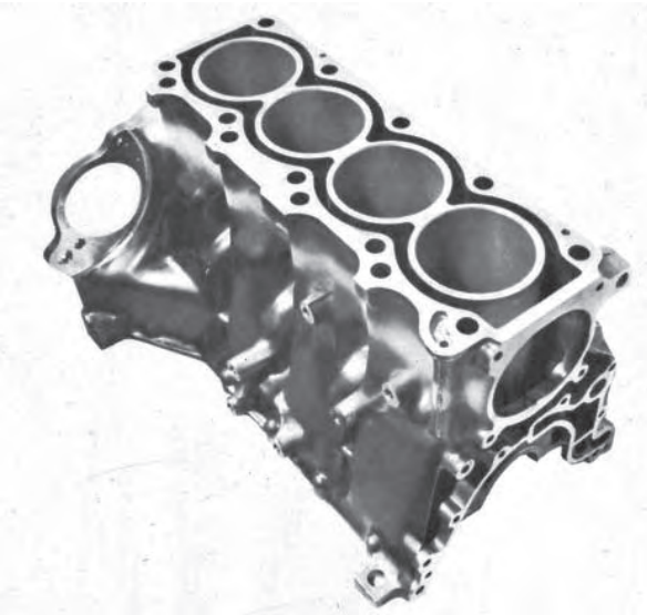
Fig. 3.47 The open-deck design, with siamesed cylinders, was adopted for the diecast aluminium crankcase of the Vega so that the dies could be easily withdrawn
