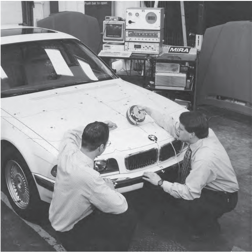
Fig. 36.9 Experts assessing the performance of a BMW bonnet when struck by a fully instrumented dummy head
