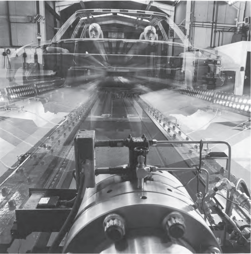
Fig. 36.6 In the MIRA impact simulation laboratory, what is in effect a giant air gun projects the sled at speeds of up to 56 miles per hour towards its target
