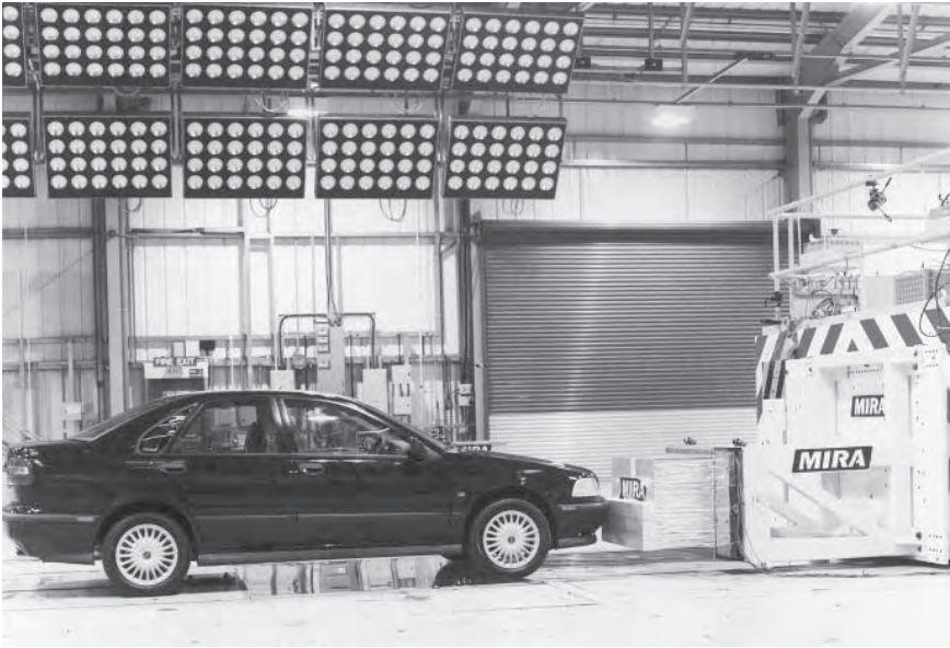
Fig. 36.3 Here a dummy front end of a car represented by an aluminium honeycomb structure is fixed to the concrete block to simulate the crushing of the other car involved in the front end impact
