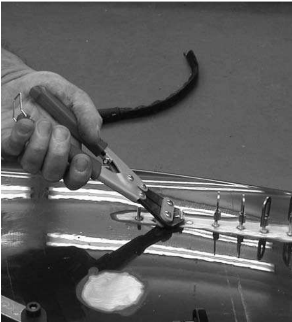
Figure 13.74 Snip-off the studs (Courtesy of POWER-TEC®)
