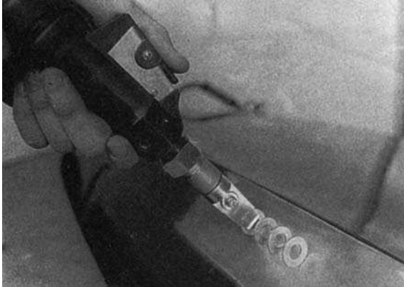
Figure 13.65 Fastening ring washers to the damaged area ready to pull ( Stanners Ltd )
