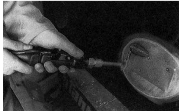
Figure 10.23 Pulse controlled roller spot welding ( Stanners Ltd )
