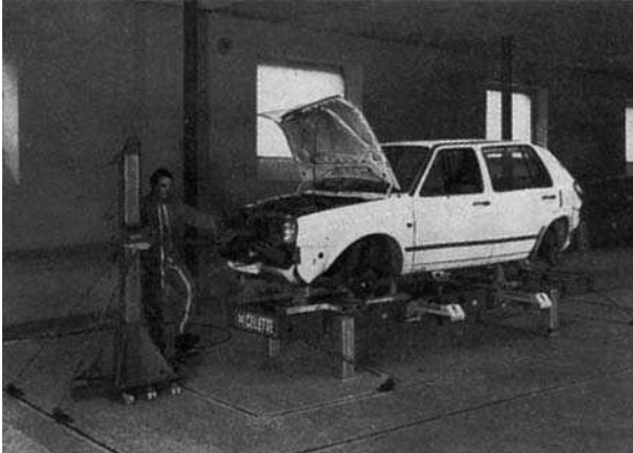
Figure 14.12 System 5000 pulling tower and frame (Celette UK)
