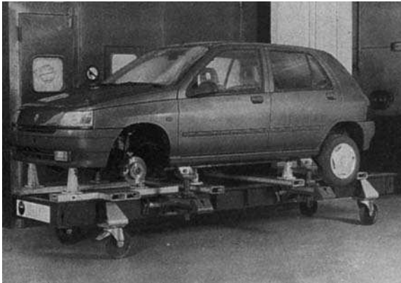
Figure 14.15 Car fixed on M8 mobile bench (Celette UK)
