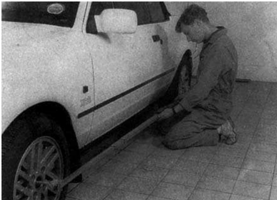
Figure 14.63 Checking a vehicle's wheel base with a digital measuring tool ( Stanners Ltd )
