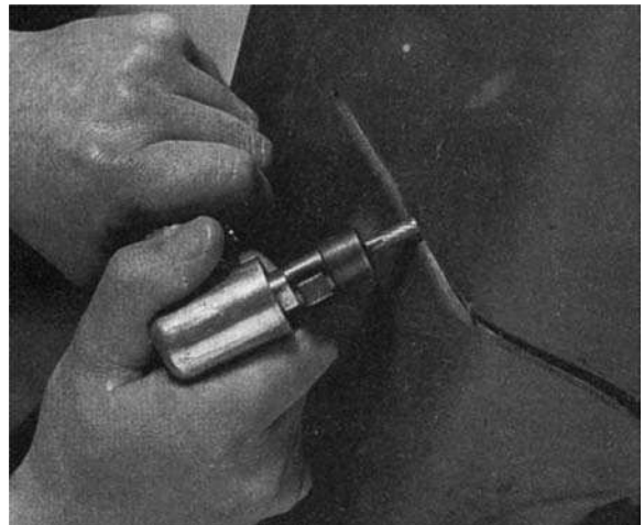
Figure 14.119 Rotary burring tool cutting a V-groove ( Welwyn Tool Co. Ltd )
