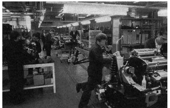
Figure 16.31 Final stages of building up chassis details on the Lotus Elan ( Lotus Engineering )
