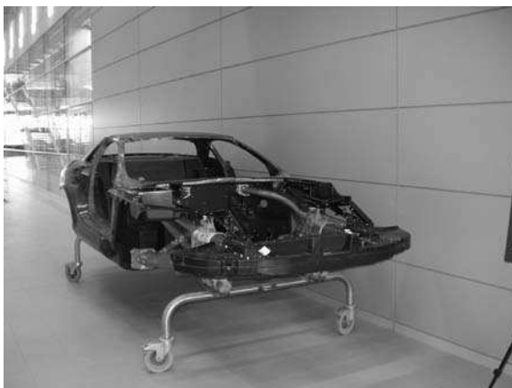
Figure 16.27 Mercedes Mchaven SLR body-in-white
