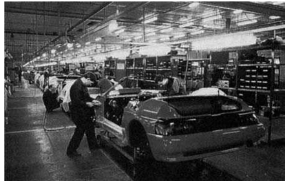
Figure 16.33 Vehicle undergoing interior trim ( Lotus Engineering )
