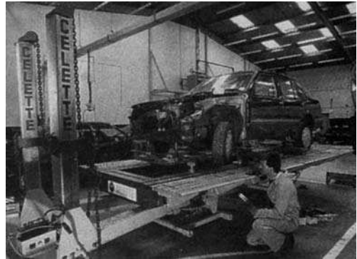
Figure 14.17 Bodymaster 2000 with Metro 2000 measurement system (Celette UK)
