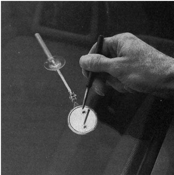
Figure 14.113 Cleaning the damaged area ( Glas-Weld Systems (UK) Ltd )
