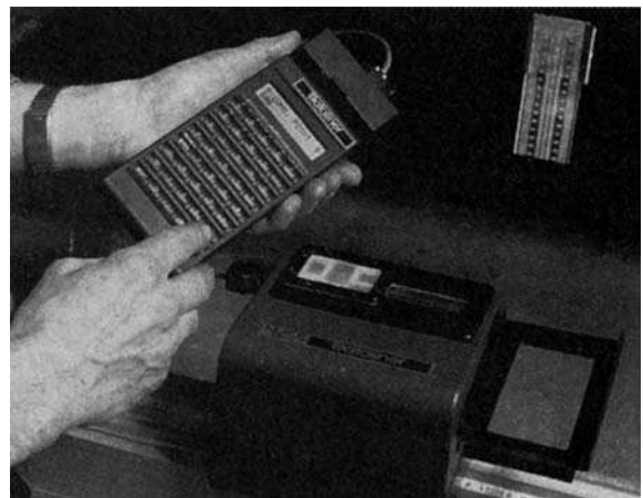
Figure 14.38 Hand-held unit with memory ( Dataliner, Geotronics Ltd )
