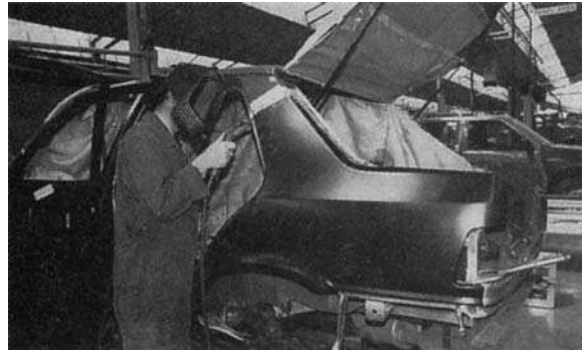
Figure 12.32 Visor-type welding screen in use ( Motor Insurance Repair Research Centre )
