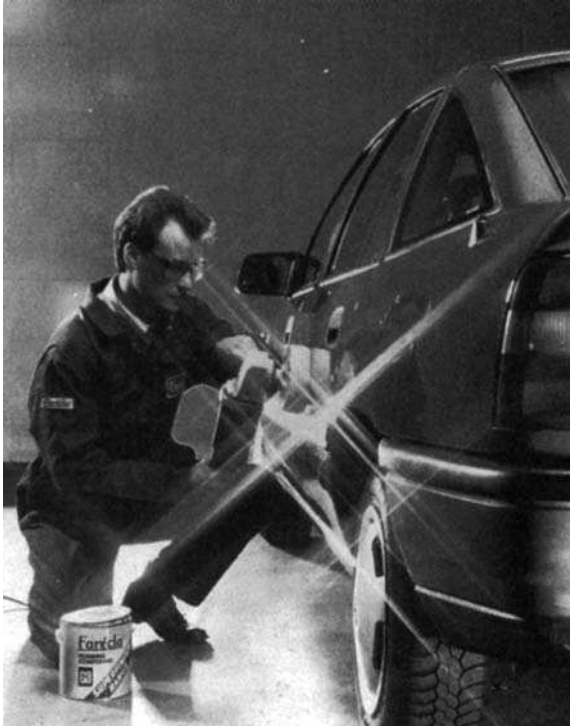
Figure 17.64 Burnishing using rubbing compound and a sponge polishing pad ( Faréncla Products Ltd )
