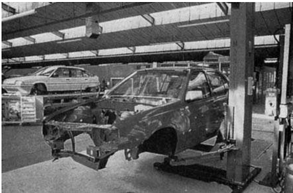
Figure 14.81 Vehicle showing front-end damage being lifted to be positioned on the jig ( Motor Insurance Repair Research Centre )
