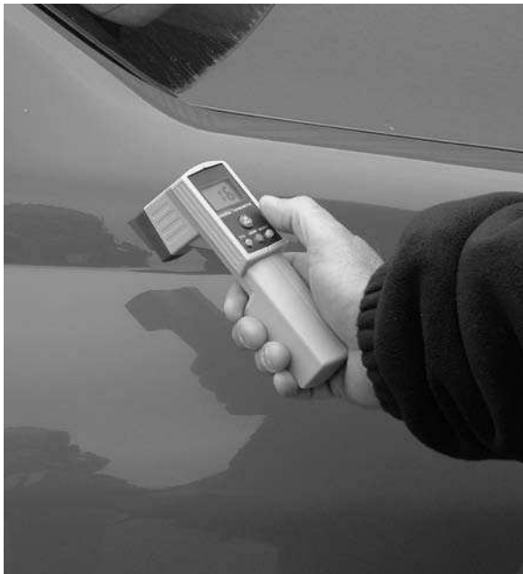
Figure 13.72 Laser point and shoot digital thermometer (Courtesy of POWER-TEC®)
