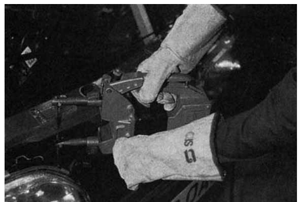
Figure 10.4 Portable spot welding machine in use (SIP (Industrial Products) Ltd)
