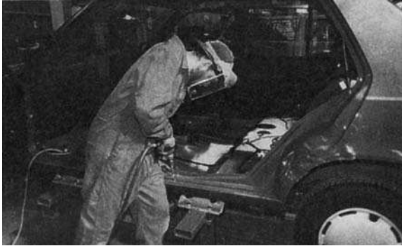
Figure 14.95 Drilling out spot welds for the removal of damaged panels ( Motor Insurance Repair Research Centre )
