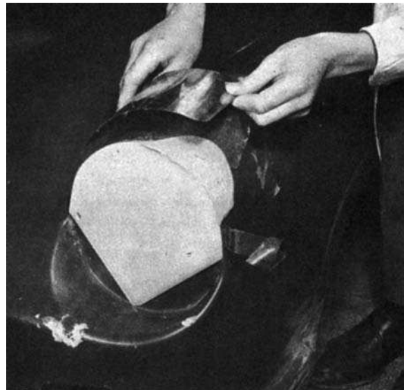
Figure 16.41 Removing temporary moulds
