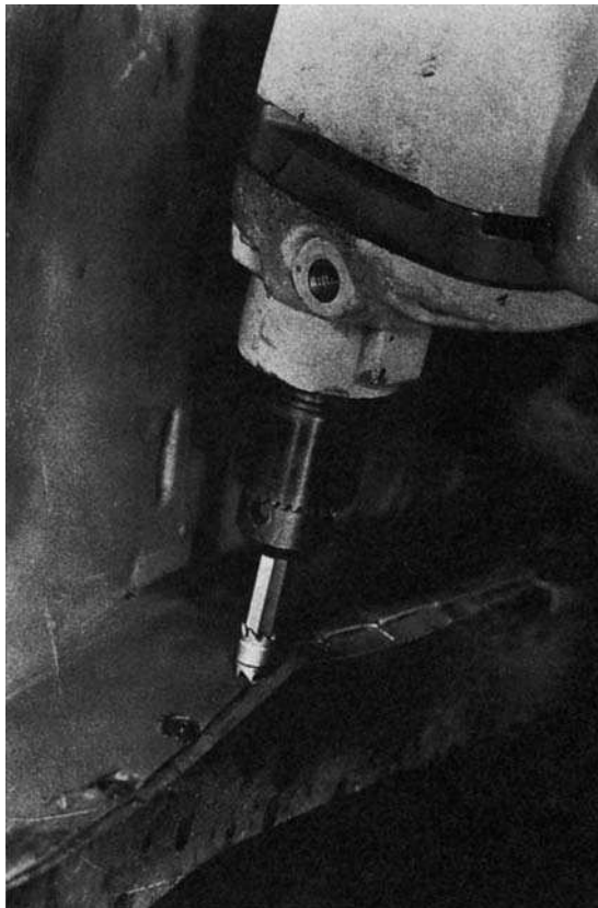
Figure 14.96 Zipcut tool for the removal of spot welds ( Sykes-Pickavant Ltd )
