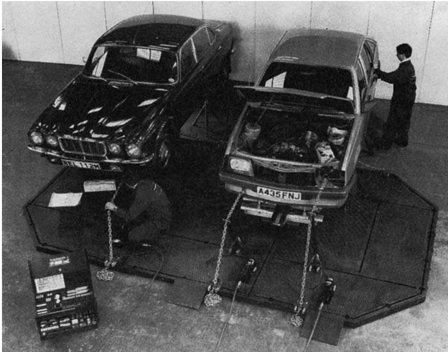
Figure 14.9 Kerek system straightening two cars at the same time ( Blackhawk Automotive Ltd )
