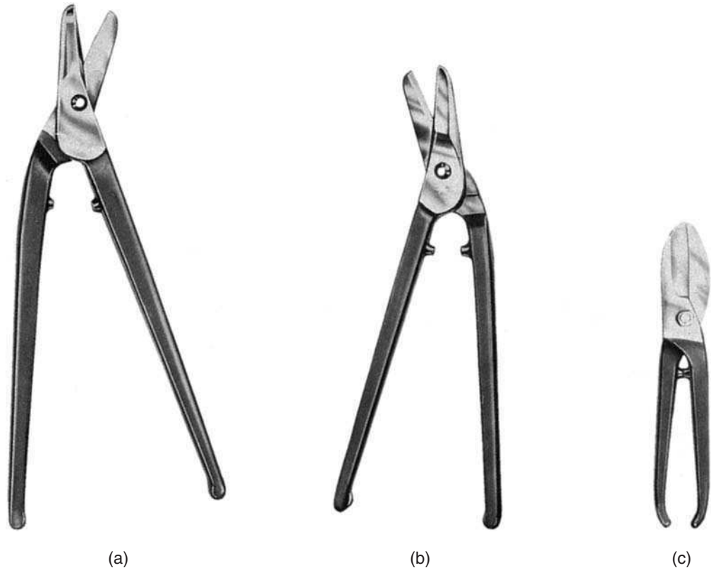
Figure 3.11 (a) Universal combination snips RH (b) universal combinations snips LH (c) standard pattern straight snips ( Sykes-Pickavant Ltd )
