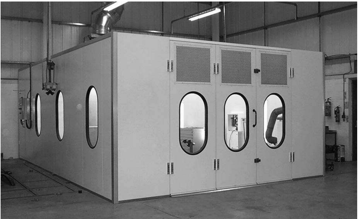
Figure 13.70 Enclosed work booth for aluminium repair ( Courtesy of POWER-TEC® )
