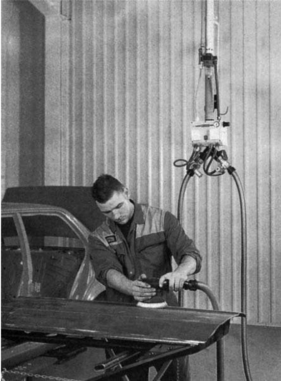
Figure 15.8 Central extraction unit ( Minden Industrial Ltd )
