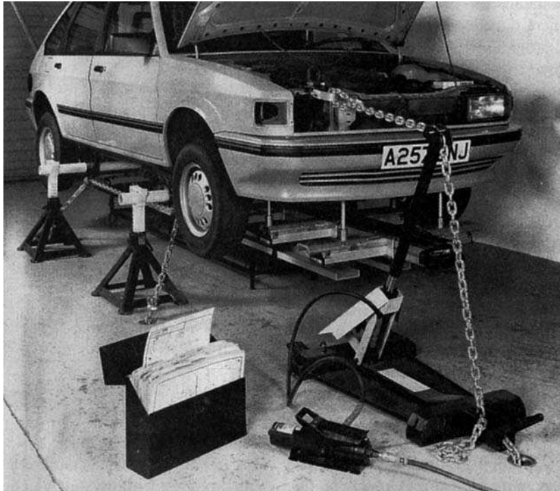
Figure 14.11 Mitek system in use, with P188 Mk2 measuring system ( Blackhawk Automotive Ltd )
