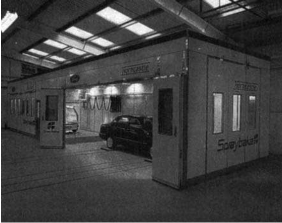
Figure 17.57 Multiple installation showing side loading doors and track, and housing IRT arch (Spraybake Ltd)
