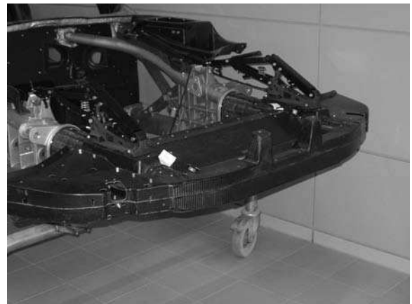
Figure 16.28 Carbon fibre composite front nose of Mercedes Mchaven SLR
