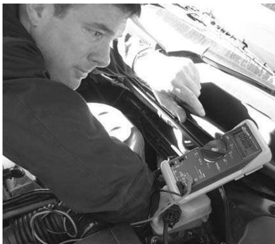
Figure 9.56 Circuit voltage testing
