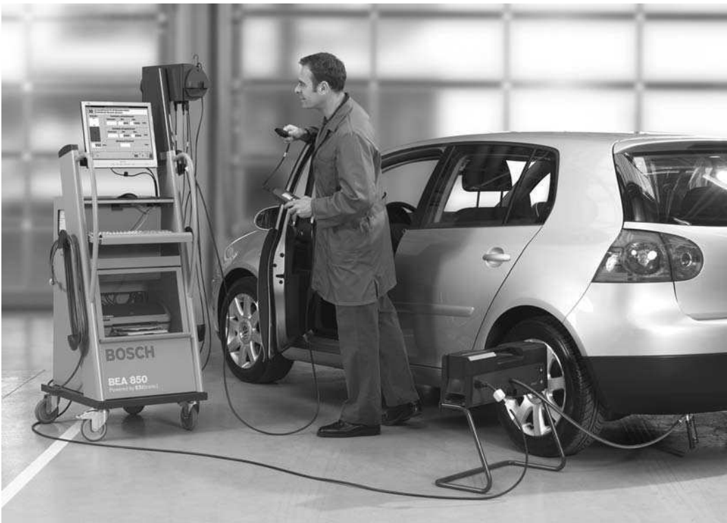
Figure 7.9 Exhaust gas analyser
