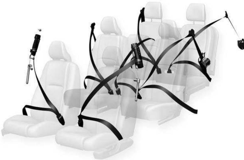
Figure 9.65 Seat belts and tensioners (Source: Volvo Media)
