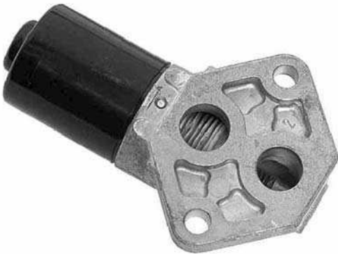
Figure 4.29 Electromagnetic idle speed control valve
