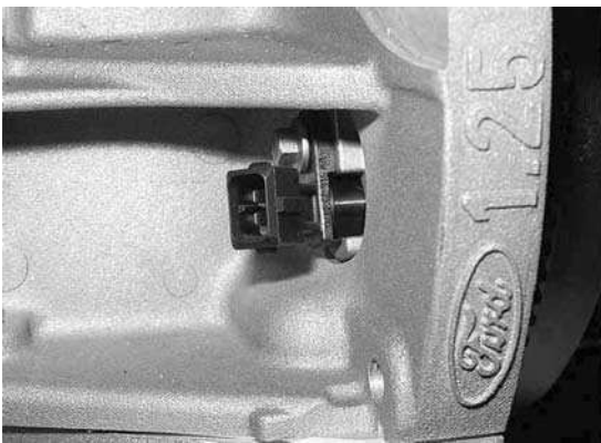
Figure 4.7 Crank sensor in position near the engine flywheel
