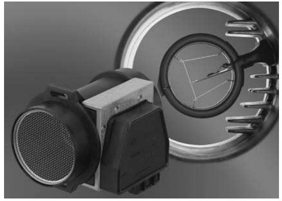
Figure 5.4 New mass airflow sensor (Source: Bosch)
