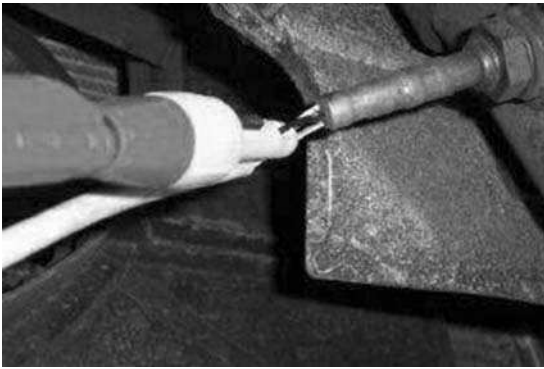
Figure 4.16 Titania knock sensor in position
