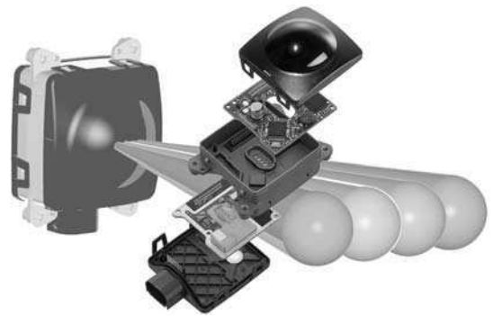
Figure 9.60 Headway sensor and control electronics
