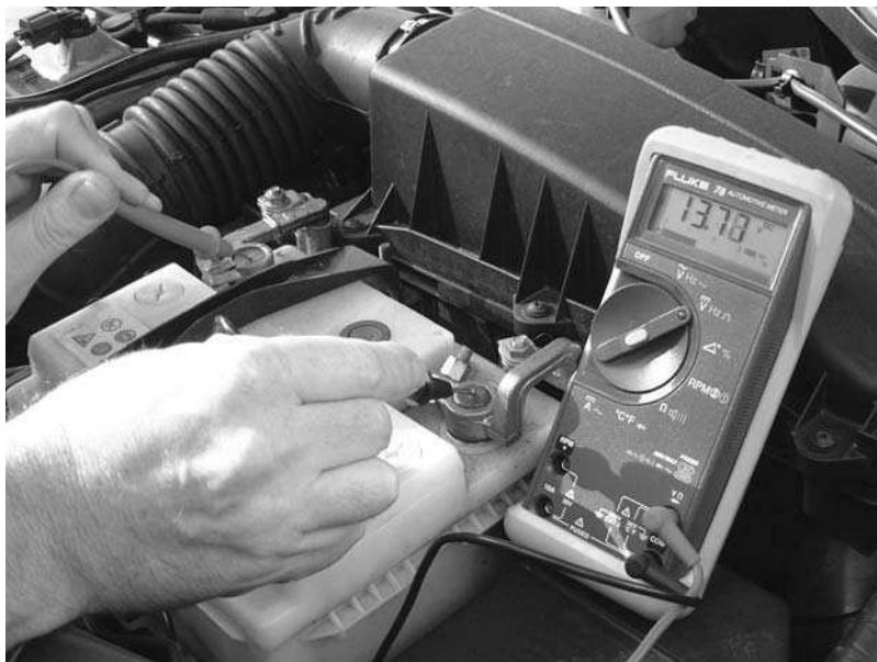
Figure 7.57 Battery voltage testing
