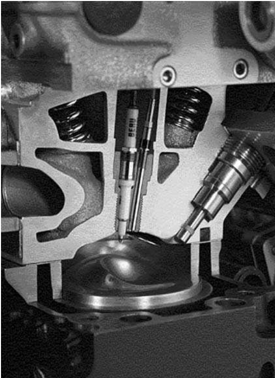
Figure 5.28 Cylinder pressure sensor mounted in the engine
