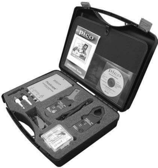
Figure 3.7 Pico Technology two-channel PC automotive oscilloscope
