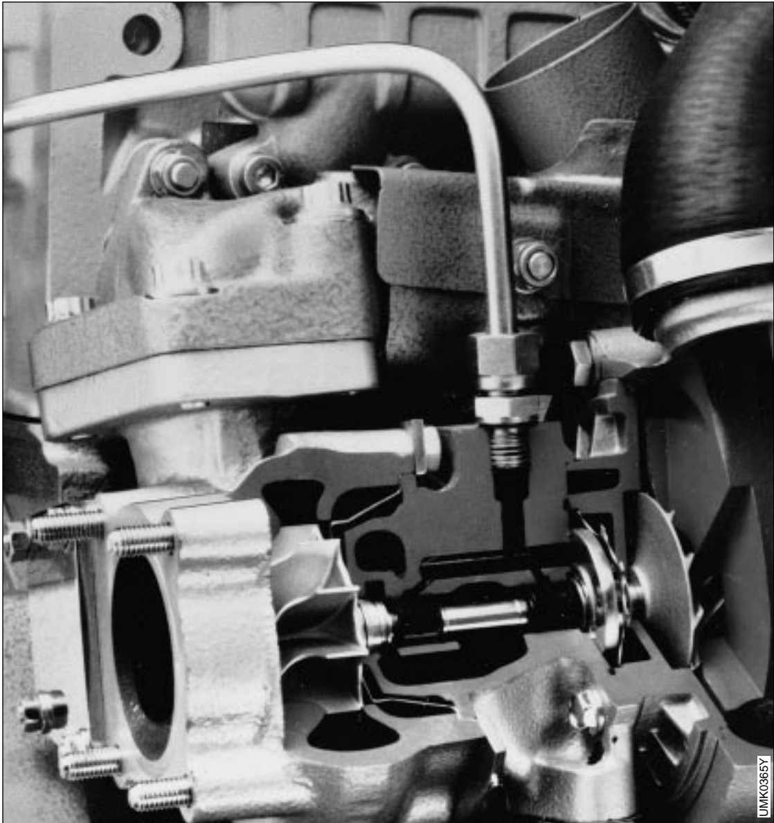
Fig. 5: Diesel engine with exhaust-gas turbocharger
