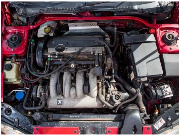
The 2.0-litre XU10J4RS engine used in the 306 GTI-6 and Rallye is unchanged between the two models and the three phases of the car's life. It's a robust unit, but with one major caveat: the timing belt.
