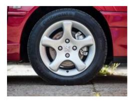
Peugeot fitted 6Jx15-inch Cyclone alloy wheels, which are cheap to refurbish and their 195/55 VR15 tyre size means there's lots of choice for those on a budget and anyone looking for stickier track day rubber. Balancing the wheels can be tricky as they don't have a centre cap, so make sure any fitter knows how to balance this type of wheel.
