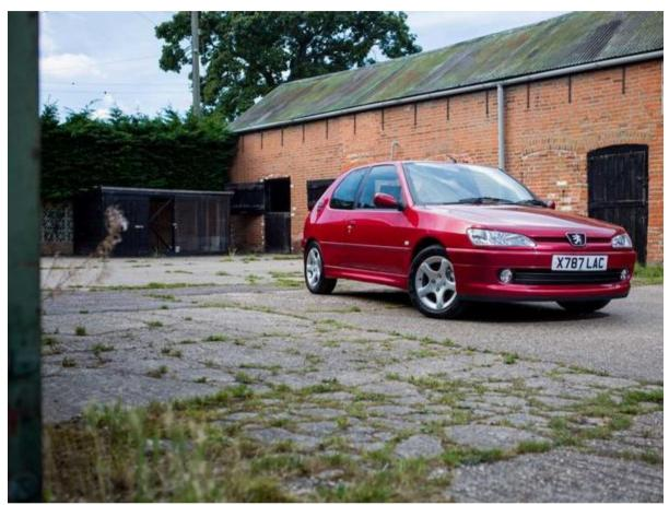
Peugeot built the GTI-6 in three phases, which can be determined from the outside. The Phase 2 revamp arrived in mid-1997 with new headlights, grille, bumpers, doors, instrument panel and side protection, while another update was applied in mid-1999. These last Phase 3 cars have 'crystal' headlights, clear side repeater indicators, round foglights, silver dash trim and an aluminium gear knob. All three phases of 306 GTI-6 have their own rear parcel shelf design.
